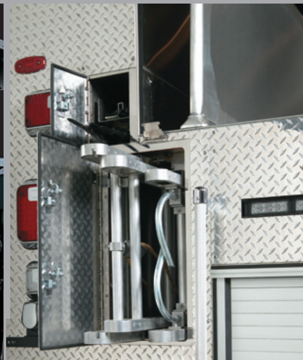
Space-saving rear folding work platform allows for easier access to the hosebed.
